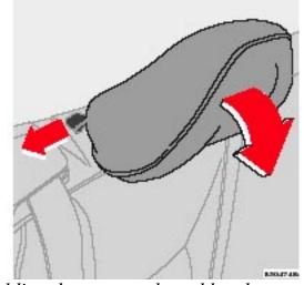
Folding down an outboard head restraint
